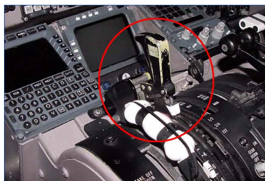
Fig 2 - Spoiler handle in the unarmed position
