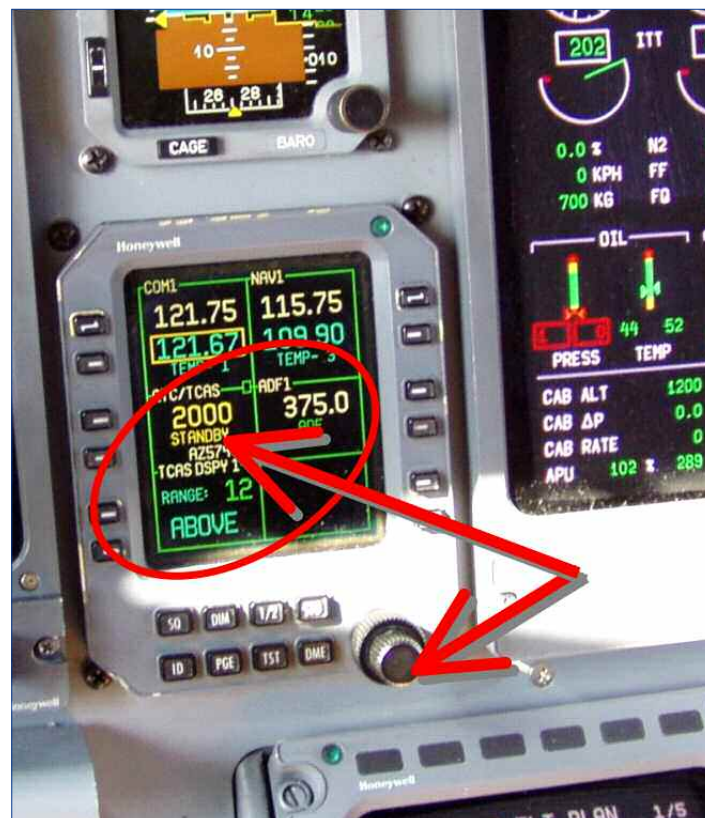
Figure 4 - Detailed view of the transponder code and mode, and the selecting knob
